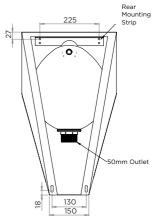
Internal waste connection can be accessed through a void in the underside of the urinal body  $\approx$  110mm x 200mm.
