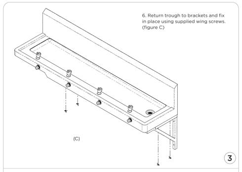
7. The trough is supplied with a 1/2 "BSP inlet to mains water.
