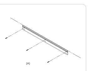
4. Place trough onto wall, hooking rear trough fold onto the joggle, suspending it from wall.
