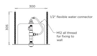
MODEL SRB Side Elevation and Plan
