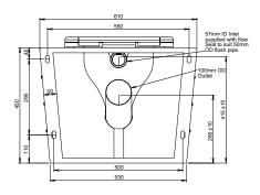
MODEL PBARRear Elevation
