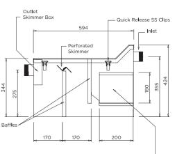
Removeable solids capture box with perforated front
