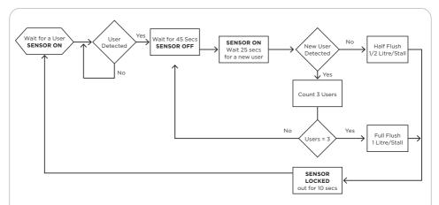
The operation of the Smart SaniFlush Sensor System (FSM) is designed to provide the most economical use of water while maintaining a clean and presentable washroom environment. It does this by only flushing once for every user if they appear in quick succession and by reducing the flush volume after one or two solitary users.
