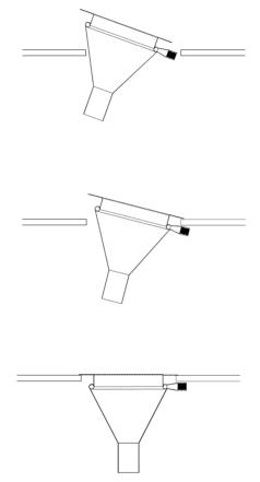
3) Place the Flushing sink into the opening according to the drawings provided above.
