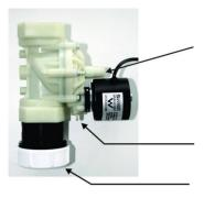
A) To lower the flow rate of the valve turn screw with a flat screwdriver in (clockwise). The factory setting is 2 turns in from all the way out. To increase the flow turn screw out (anticlockwise).
