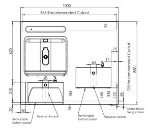
MODEL DDR2-HFBF Front Elevation
