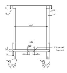
MODEL BT-MB-612 Front Elevation
