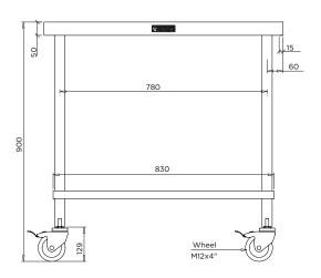
MODEL BT-MB-609 Front Elevation
